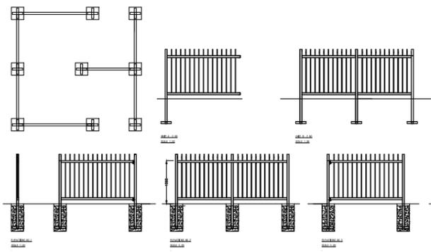
H) Chicane with Blunt top panels colour to be powder coat Green. Height of panels to be 1.2 metres high.
